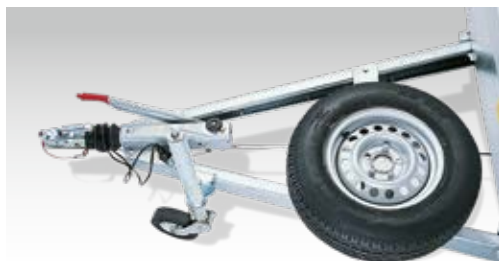
Spare wheel bracket mounted on the drawbar (only possible on long drawbars and certain models)
