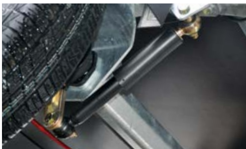
Wheel shock absorbers (mounted), with 100 km/h confirmation; wheel shock absorbers (loose) without 100 km/h confirmation
