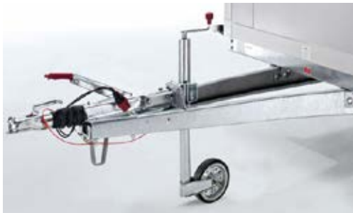
Long drawbar (version depends on model)
